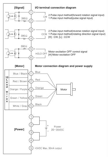
Add external resistor when power for pulse from the external of the unit exceeds +5VDC
